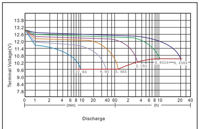
★ The above are average and date obtained from the first 3 charge/discharge cycles. These are not minimum values.
